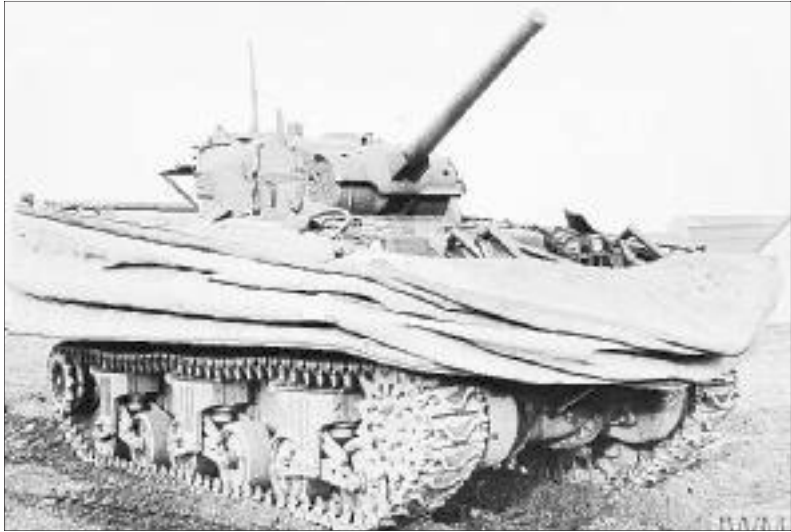
Two of 'Hobart's Funnies,' a tank that could swim ashore like a duck and a tank that flailed away at hidden landmines.
